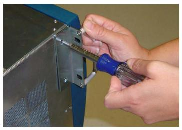
Figure 2-1: Install the Rack Ears on the Chassis
